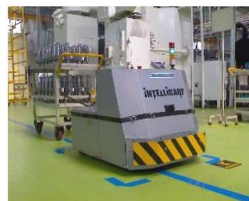
Figure 2: AGV guided by a line on the floor
