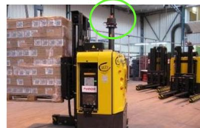
Figure 3: AGV guided by a laser
